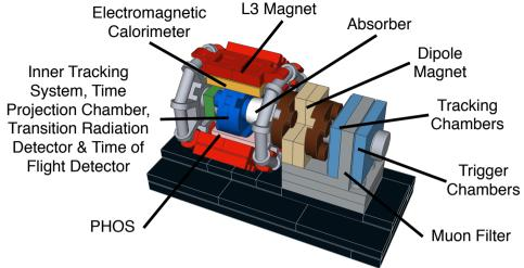
ALICE is a heavy-ion particle detector at the Large Hadron Collider (LHC) in CERN, which has been designed to investigate an exotic state of matter known as a quark-gluon plasma. The LHC spends a few weeks each year smashing lead nuclei together, causing their protons and neutrons to melt and recreating conditions that existed a fraction of a second after the Big Bang.
